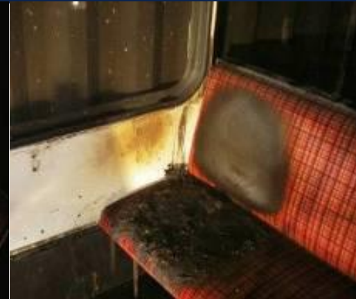
Full Scale Fire Test with Activation of FOGTEC System
