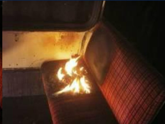
Full Scale Fire Test with Activation of FOGTEC System
