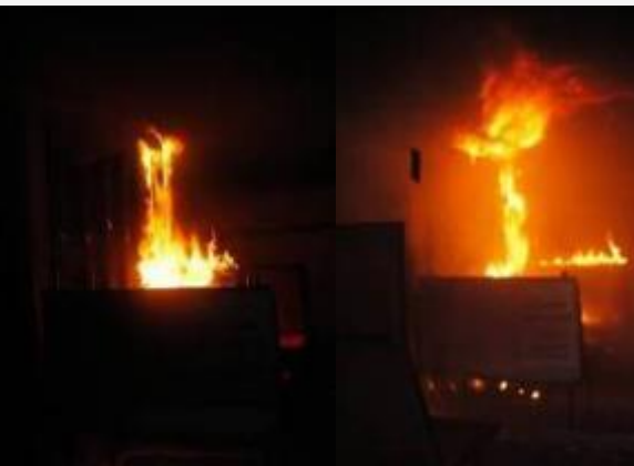
Full Scale Fire Test without Activation of FOGTEC System
